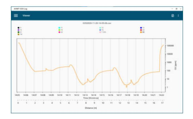
**Precise** measurement from percentage to ppm level to recognize root cause of voiding
