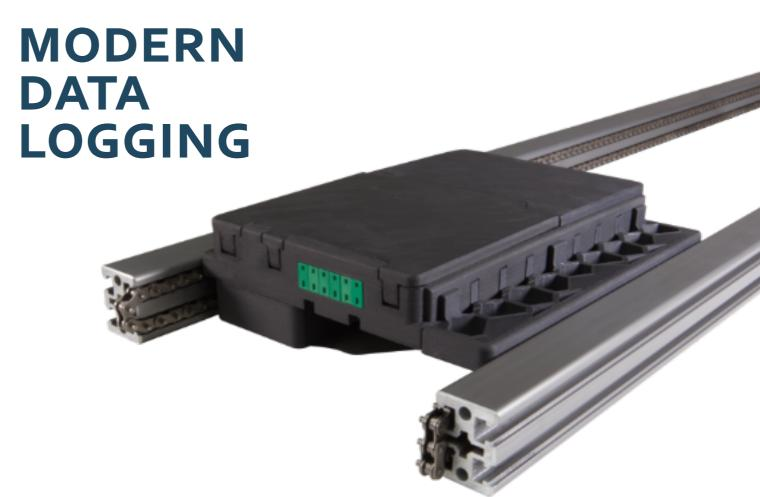
The AHMT Omnibus data logger enables total process control of reflow lines to increase yield and quality of the production. The wireless system measures temperature, atmosphere and multiple mechanical settings of the oven and the previous as well as post processes.
